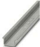
DIN rail, unperforated, acc. to EN 60715, material: Steel, galvanized, passivated with a thick layer, Standard profile 2.3 mm, color: silver
