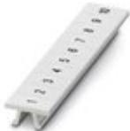
Zack marker strip, Strip, white, labeled, printed horizontally: consecutive numbers 1 ... 10, 11 ... 20, etc. up to 491 ... 500, mounting type: snap into tall marker groove, for terminal block width: 5.2 mm, lettering field size: 5.15 x 10.5 mm, Number of individual labels: 10
